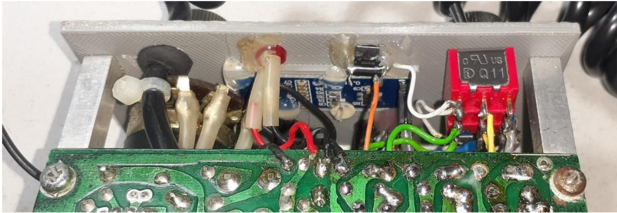
Figure 7 : The lower section of the Band switch wiring as well as the Lock switch and OLED mounting can be seen here.
