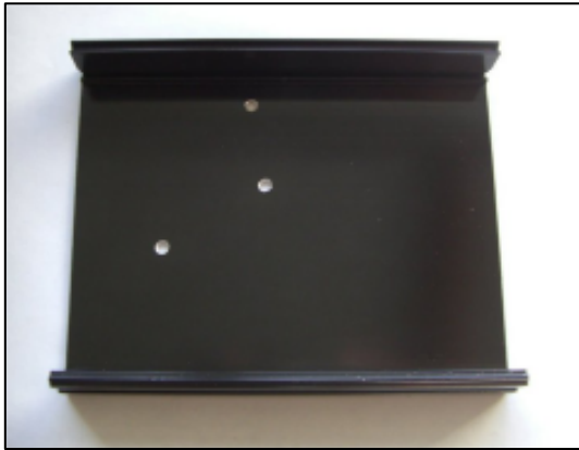
Figure 17: One half of the enclosure has been drilled and is ready to mount the PCB
