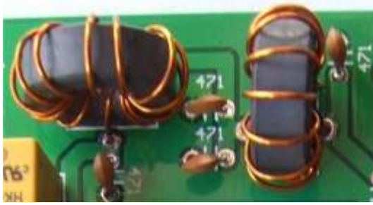
Figure 13: Completed toroid coils L6 and L7 installed in the transceiver PCB
